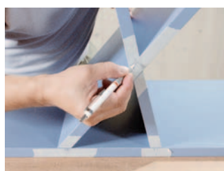
2. Copy the centre to the second workpiece
