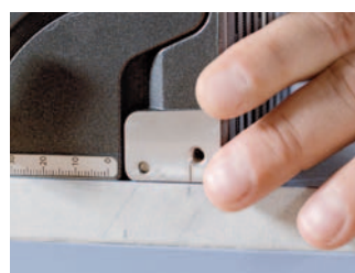
3. Align the Zeta P2 with the marking
